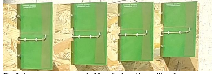
Fig. 3. Antenna array composed of four dipoles with metallic reflectors.
